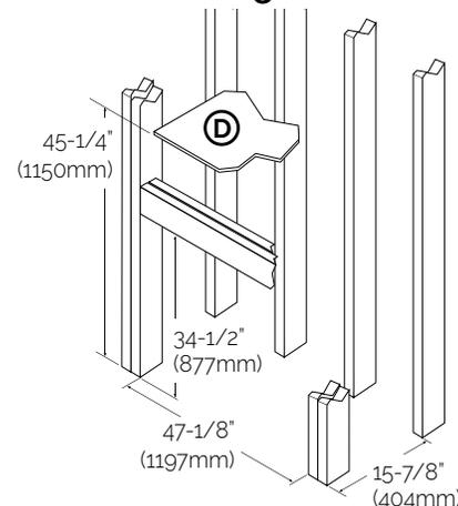
**D** The fireplace enclosure must be a minimum 45-1/4" (1150mm) tall. Do not build into the fireplace enclosure.
